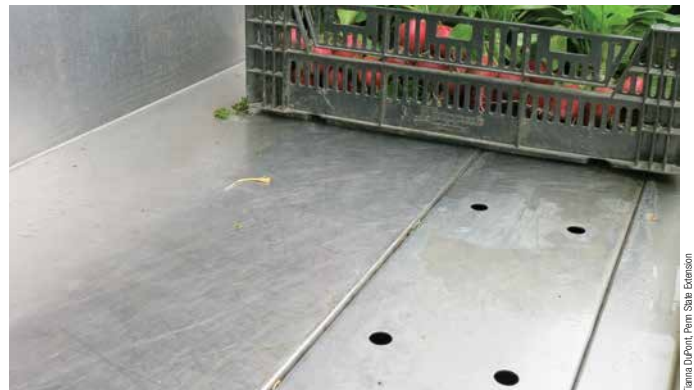
The holes in the table move water into a channel under the table and into a drain that is away from workers' feet. Stainless steel makes it easy to clean and sanitize.
