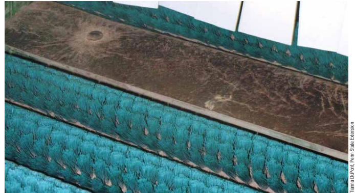
The nooks and crannies in packing equipment can harbor pathogens. Make sure to have a policy and schedule for frequent cleaning and sanitizing.
